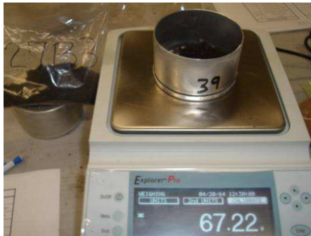
Fig. 7: Wood Sample for Moisture Content Testing
