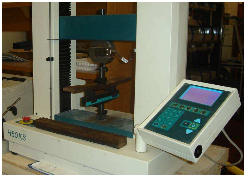
Fig. 6: Ultimate Strength Testing of Specimens
