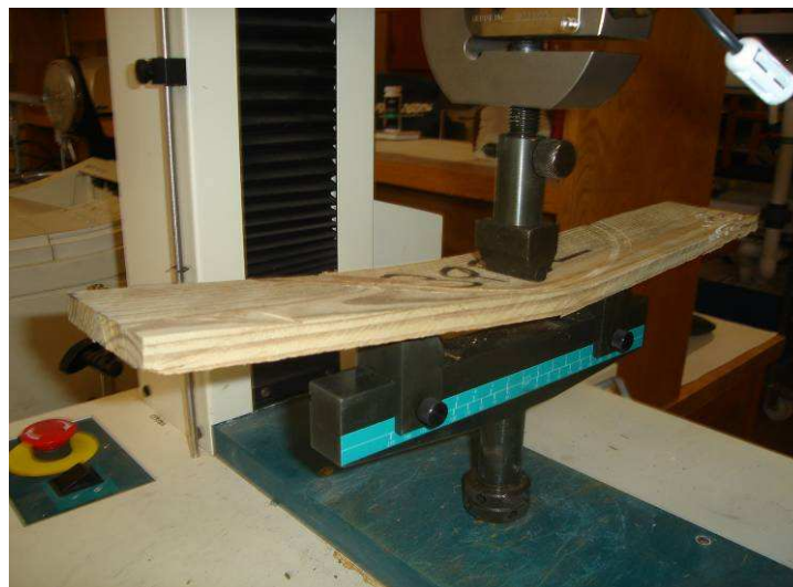
Fig. 9: Three-Point Bending Testing
