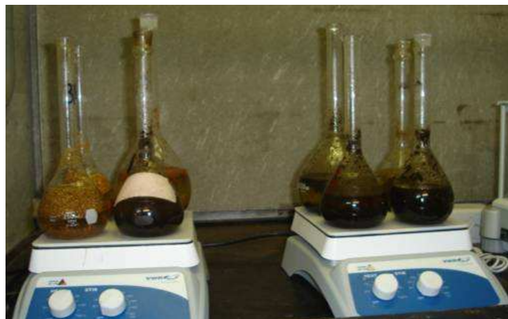
Fig. 8: Boiling of Wood Samples in Volumetric Flasks
